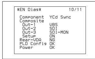
**Component:** Setting status of the component output signal from the OUTPUT connector and status of the sync signal added to the component Y/G output signal from the OUTPUT connector
